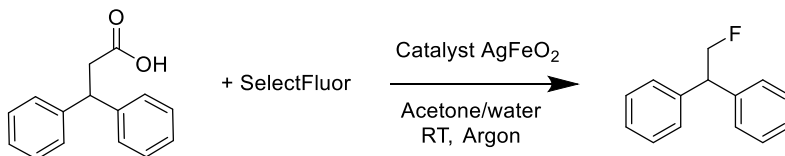
Scheme 0.2. The fluorination of 3,3-diphenylpropionic acid with SelectFluor to afford (2-fluoroethane-1,1-diyl)dibenzene using \text{AgFeO}_2 nanoparticles as catalyst
